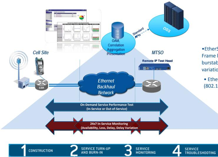
•EtherSAM Y.1564 for Turn-up Frame loss, delay, throughput, burstability, frame delay variation
